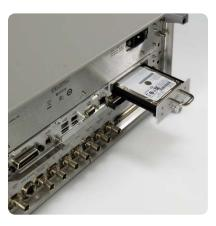
An upgradeable CPU module (left) lets you easily achieve faster processing and interface speeds and a removable hard disk drive (right) simplifies instrument sharing and ensures data security.
